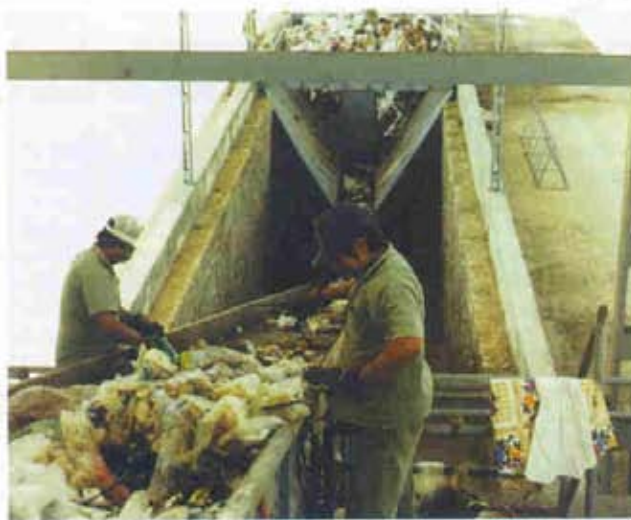
The inability to remove all contaminants from incoming feedstocks resulted in low quality composted products.
